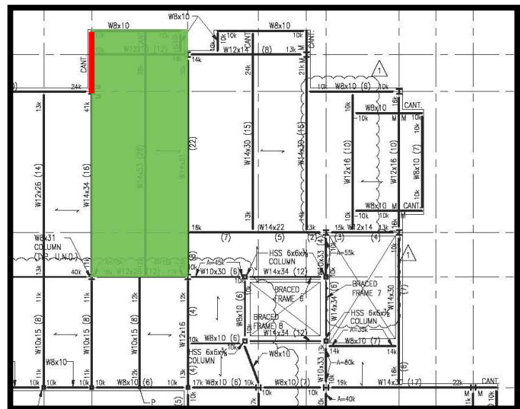
Figure 19. Cantilevered Beam G.B-G.11
